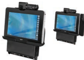
LOCKING MOBILE DOCK 509.056.00 • Full port replication • Available with locking mechanism • Compatible with SlateMate™ tablets
